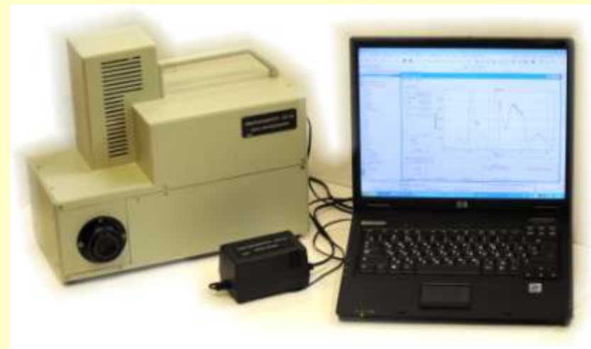
Spectroradiometer ПСР-02 (spectral density of energy brightness and the polarization characteristics of radiation )
