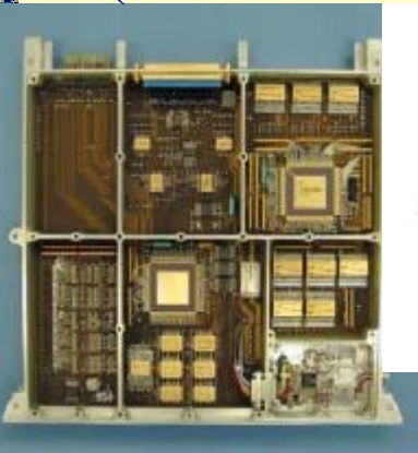
Control System (GNSS/GPS Receiver)
