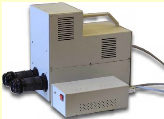
Spectrometer PVS-02 ( the emission, reflection and absorption spectra)
