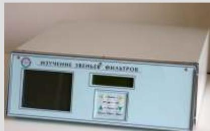
The facility makes it possible to study the properties of four types of filters: low and high frequencies filters and band-transmission and band-stop filters, as well as resonance amplifier. The graphical display builds amplitude and frequency and phase-and-frequency characteristics.
