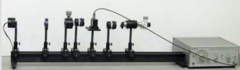
As an ultrasonic source a piezoelectric based on  $\text{BaTiO}_3$  has been taken with eigenfrequency in the range 1-10 MHz. The accuracy of output signal frequency maintenance makes  $\pm 2.0\%$ , source voltage amplitude is 5.0 - 30.0 V. The work makes it possible to examine the diffraction pattern changing at changing the structure of phase grating and to specify the period of grating.
