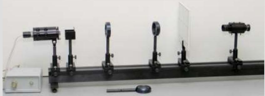
The work is aimed at experimental verification of the basic laws of geometrical optics. It allows to determine lenses focus distances, principle and focal planes of converging and divergent lenses and optical systems (the error does not exceed  $\pm 5.0 \cdot 10^{-3}$  m), their spherical and chromatic aberrations.
