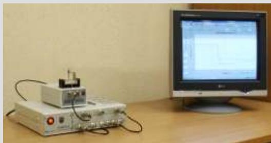
The module of non-stationary LCR-spectroscopy
