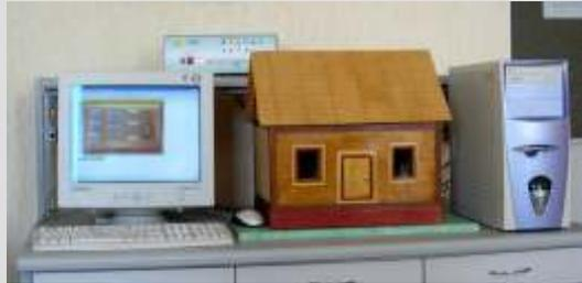
The system is intended for experimental laboratory works for training of the 4<sup>th</sup>-5<sup>th</sup> year and master students by the energy saving principles, examination of the heat transfer characteristics in closed capacities, measurements of thermal characteristics
