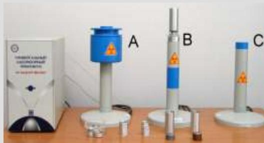
The use of detecting unit with unlimited scintillator with a set of lead and copper absorbers and gamma-sources and a set of low-active volume sources enables to carry out five laboratory works ( ).
