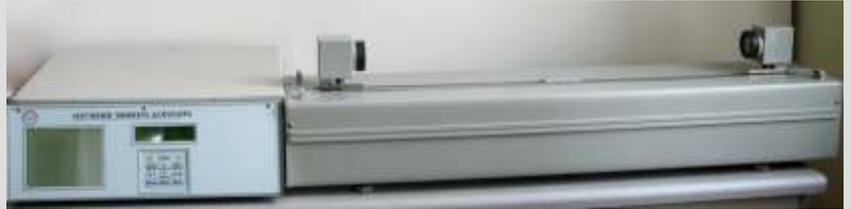
Ultrasonic wave propagation in air is studied. Damp coefficient is determined. The work provides the movement of the receiver and the radiation source which enables to check the theory of Doppler's principle.
