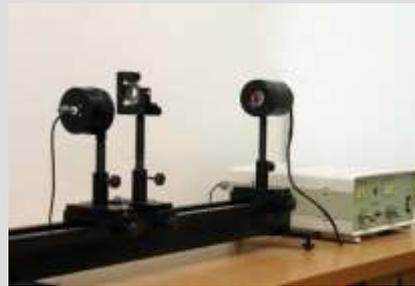
The device enables to measure volt-ampere characteristics of a photoelement at accelerating and arresting voltages, to determine the accelerating voltage value (measurement accuracy
